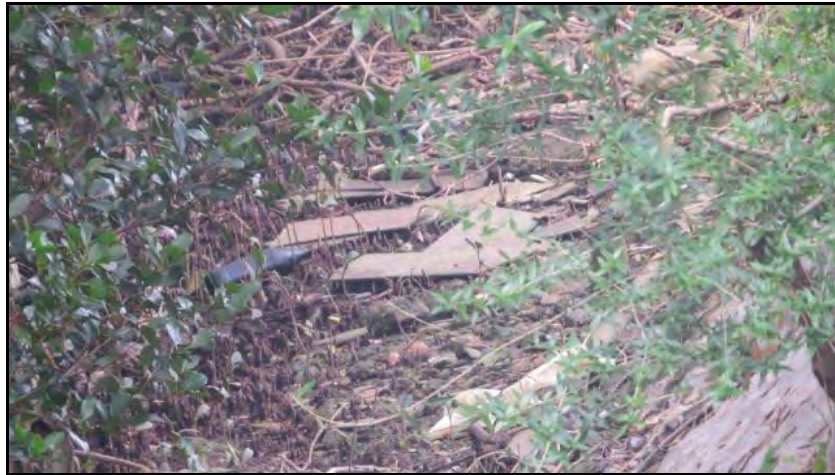
Photograph 2E: The sheets of asbestos cement are visible through portions of this fabric.
